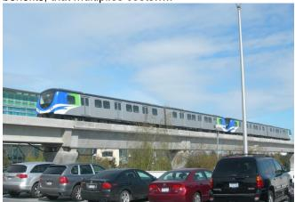
A *Skytrain* is automated. It has no driver. This requires traffic separation, either on elevated ways or in tunnels, with a cascade of negative consequences:
